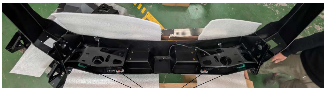
OEM sensor holder (bonded with double-sided tape)
